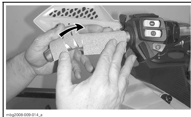
TYPICAL — CORK INSULATOR ALIGNMENT
