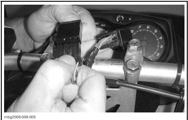
TYPICAL — STEERING CONNECTORS
